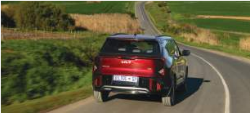
Lane Following Assist Keep the vehicle centred in its lane with gentle steering support when lane markings are detected. *Available on GT-Line S and X-Line models.
