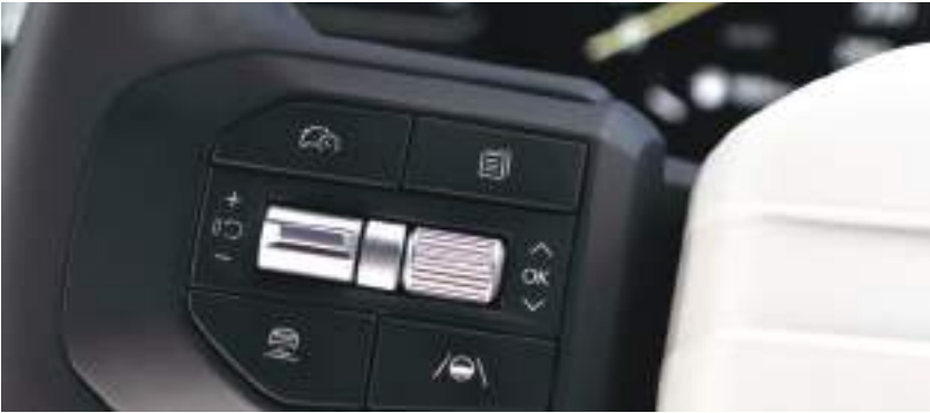
Smart Cruise Control with Stop & Go Maintain a set speed and following distance from the vehicle ahead, with Stop & Go functionality that helps reduce driver effort in slower-moving traffic. *Available on GT-Line S and X-Line models.
